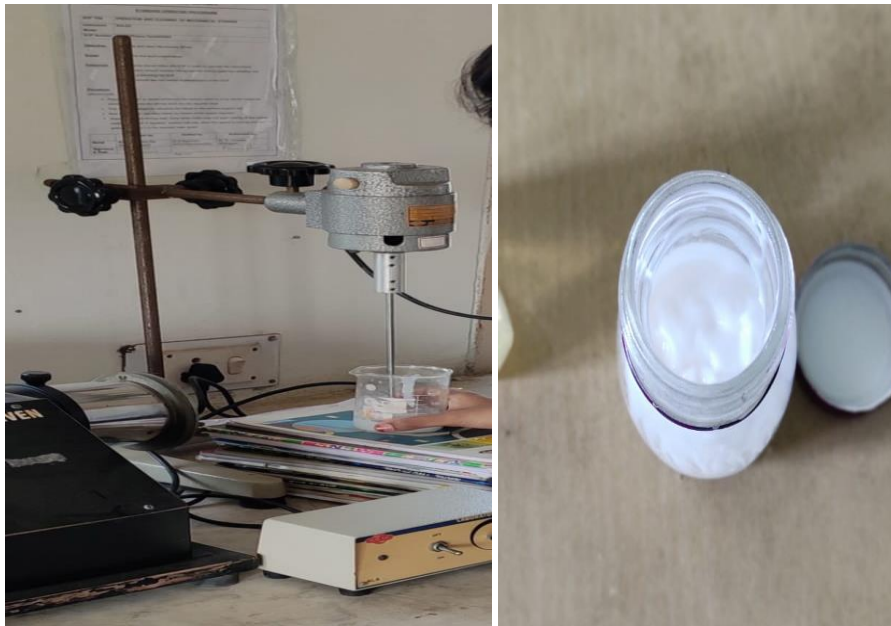
Fig: Formulation of emulgel using mechanical stirrer.
