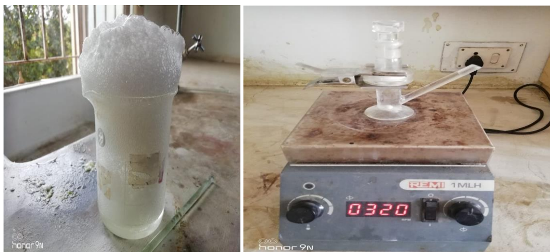
Fig: Preparation of egg membrane and in vitro diffusion study using Franz diffusion cell.
