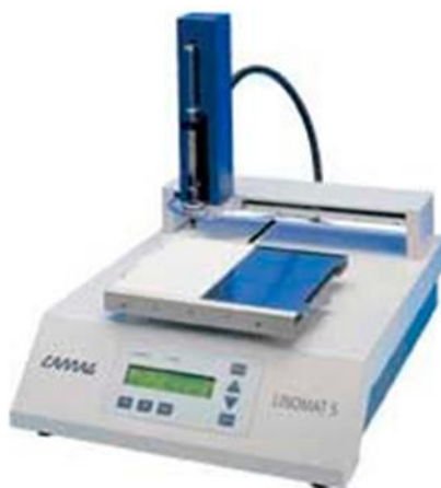
Figure 2: Camag Linomat 5 Sample Applicator used in HPTLC.
