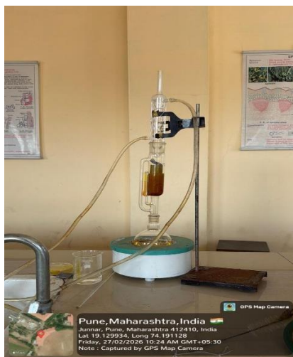
Fig. 1: Curcumin Extraction Process.
