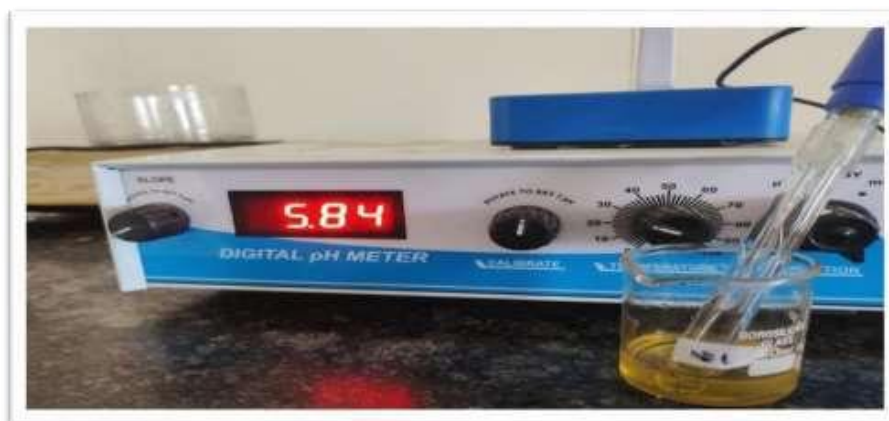
Fig. 9: pH measurement of Microemulsion.
