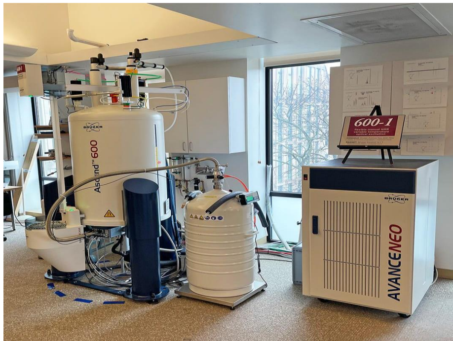
Figure 11: Instrumentation Layout of a High-Resolution Bruker Avance NEO 600 MHz Superconducting NMR Spectrometer.
