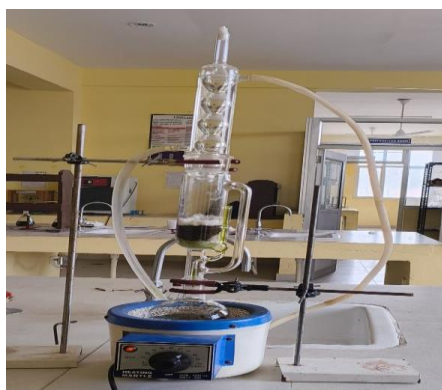
Fig. 3: Extraction process by Soxhlet apparatus.
