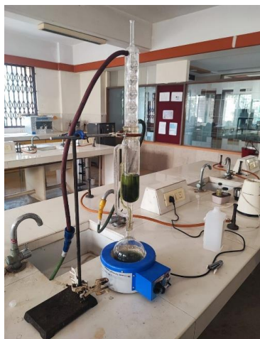
Fig.1: Extraction of Eugenol from piper betle leaves using Soxhlet apparatus.
