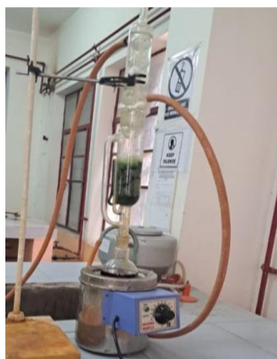
Figure No. 2: Soxhlet extraction process.
