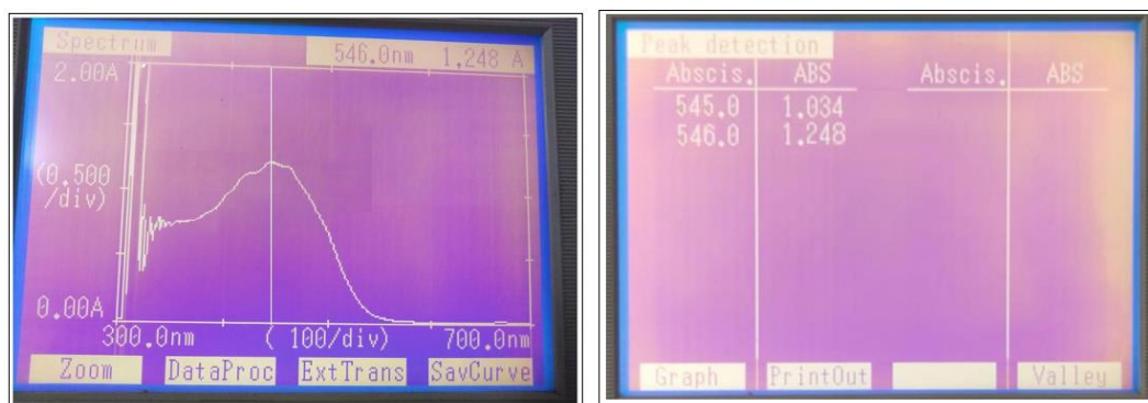
Fig 5: Absorbance maxima of Mangiferin at 546.0nm by nitric oxide (NO) method.
