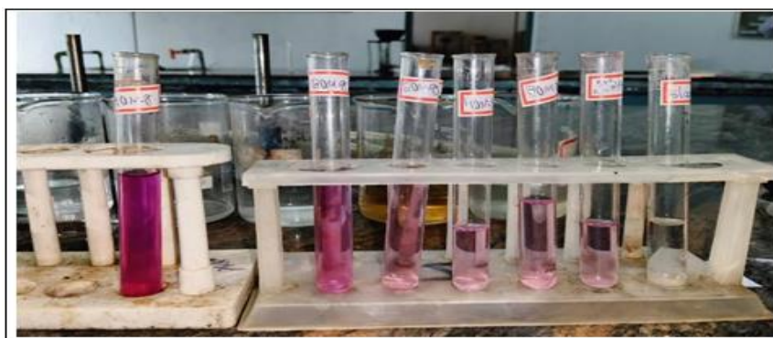
Fig 4: Colour Chromogen of Ascorbic acid and Mangiferin by nitric oxide (NO) method.
