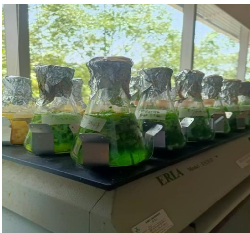
Figure 3: Maceration process of the mixture in the orbital shaker for seven days.
