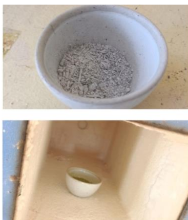
Fig. 3: Determination of ash value using muffle furnace.
