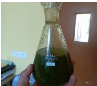
Fig. 4: Extraction by Cold Maceration Method.
