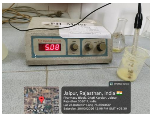
Figure No. 5: pH measurement of prepared cream.
