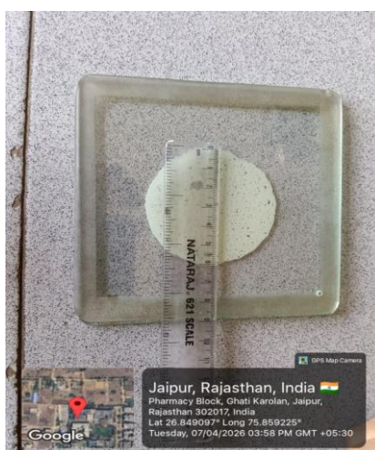
Figure No. 7: Cream applied between 2 glass plates for measurement of spreadability.
