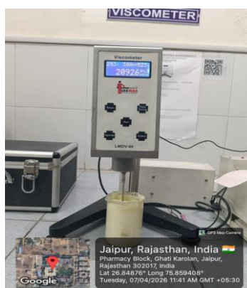
Figure No. 8: Viscosity measurement by Brookfield viscometer.
