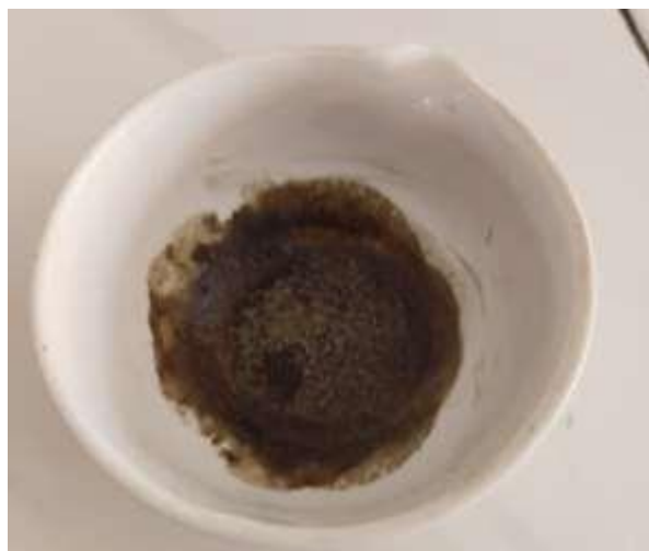
Figure 5.4: Solid content test showing dried residue of formulated herbal shampoo after water bath drying.
