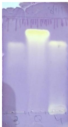
Figure 10: Chromatogram of antioxidant activity after spraying with mixture (DPPH). Elution system: ethyl acetate/formic acid/water (8/1/1); 3: methanolic extract; 4: aqueous extract and Q: quercetin.
