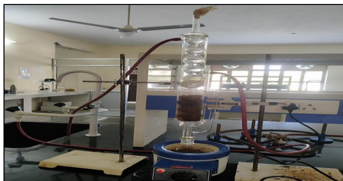
Figure 5.1: Extraction assembly of cinnamon.
