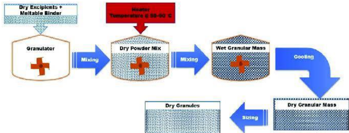
Melt Granulation – Schematic Diagram
