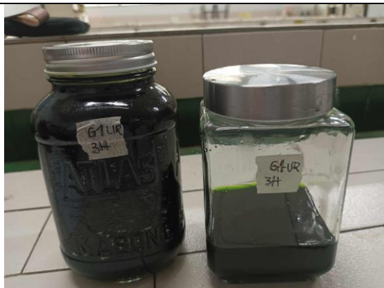
Image 4: Maceration. The powdered leaves were soaked in an adequate amount of 80% methyl alcohol, ensuring complete submersion. Plant sample was macerated for a period of 24 to 48 hours.
