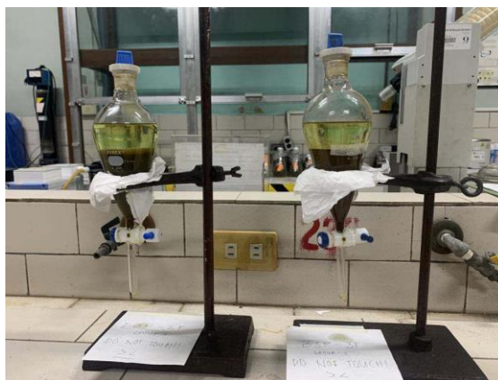
Image 5: Solvent Partitioning. Using solvent fractionation, the methanolic extract yields aqueous, ethyl acetate, and hexane fractions.
