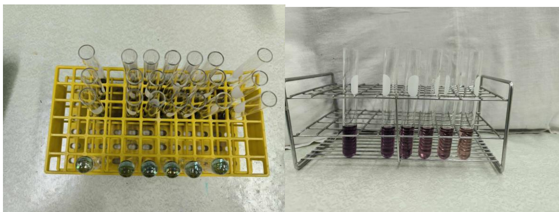
Image 7: Different concentrations of the sample were mixed with 5 mL of 0.1 nM DPPH solution.
