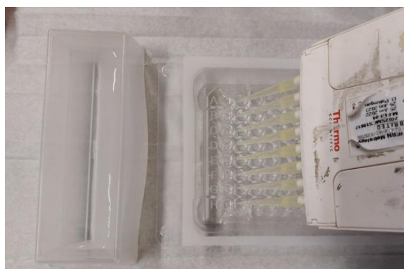
Image 14: Dispensation of 180uL PBS buffer pH 8.0 into the 96-well plate using a multichannel pipettor.
