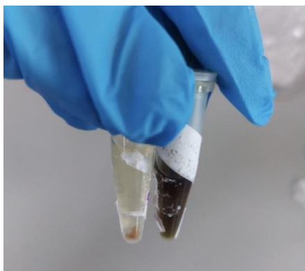
Image 13: Preparation of samples. Sample on the left was only partially soluble to solvent while the right was completely soluble.
