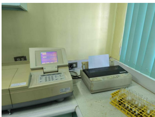
Image 8: The absorbance of the reaction mixture was measured at 517 nm using a double-beam UV-Vis spectrophotometer.
