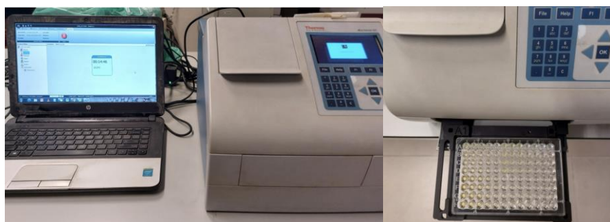
Image 17: (Left) Incubation of well mixture for 15 minutes using Multiskan (Thermo Scientific). (Right) Dispensation of 15uL substrate (acetylcholine iodide) into the 96-well plate after the incubation.
