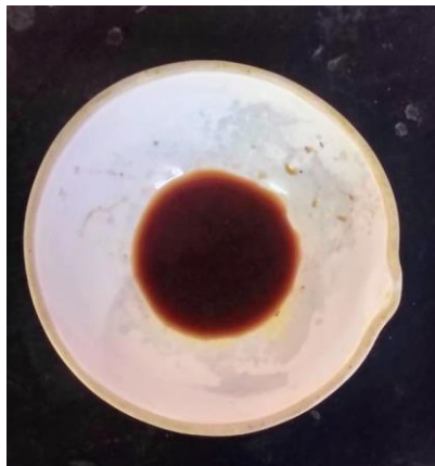
Fig. 11: Ferric chloride test — tannins ( Syzygium cumini ).
