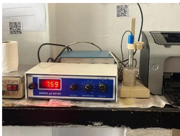
Fig. 12: pH determination of the formulated toothpaste.
